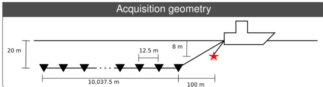
Streamer (length 10 km) record P-waves in the water
