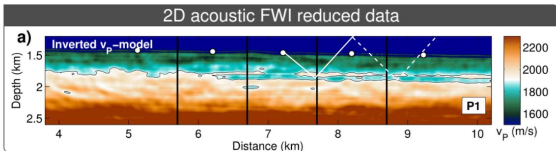
→ Artefacts are removed when using reduced data
