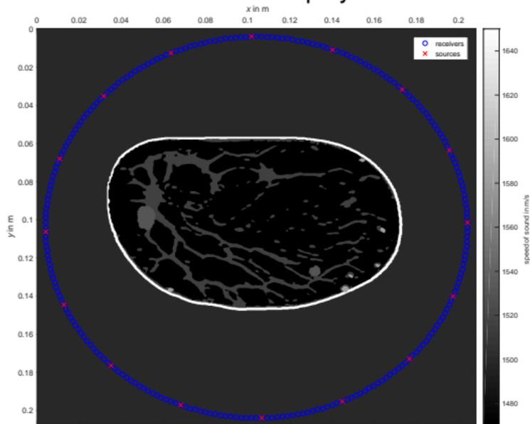
2D acquisition geometry used in the reconstruction test.
